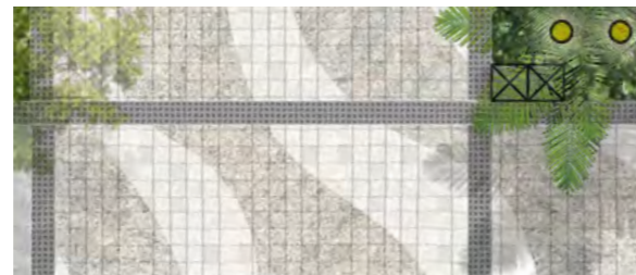
Feature Paving: Juperana Stretcherbond Pattern
